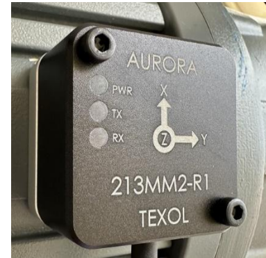
Figure3-9 Successfully Mount 213MM4-R0 Digital Multivariable Sensor
