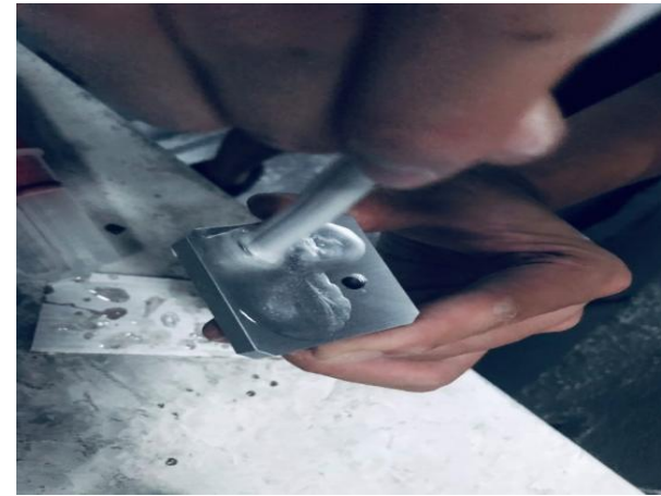
Figure3-5 Applying AB Glue onto Base
