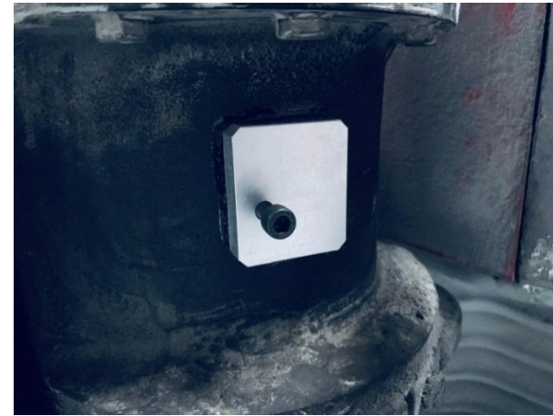
Figure3-7 Waiting for AB Glue Curing
