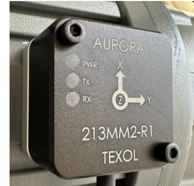
Figure3-24 Successfully Placed 213MM2-R1 Smart Sensor
