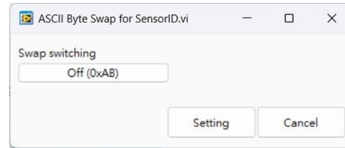
Figure3-66 Aurora Modbus Utility Device ID ASCII High/Low Byte Function Selection
