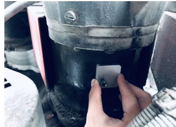
Figure3-21 Fixing Base on Equipment Surface
