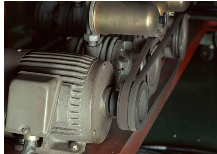
Figure2-4 Motor Drive End - Belt Drive
