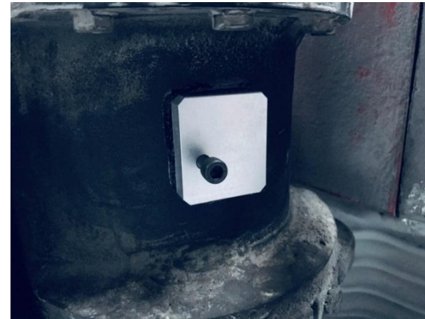
Figure 3-7 Waiting for the AB Epoxy to Cure
